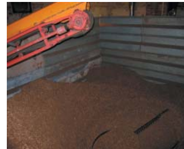
potato elevator and revolving arm auger feed
