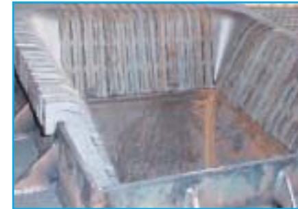
The underfed hearth system (courtesy Stewart Thermal Ltd)
