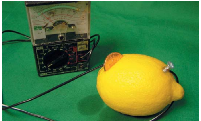
Using a voltmeter we measured our lemon generating a whopping four volts
